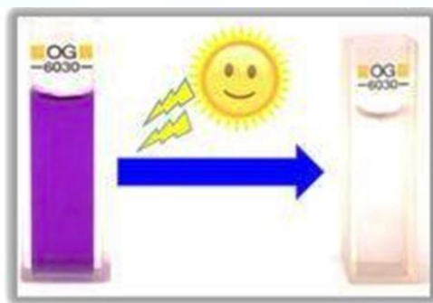
Figure 1: Photographic image of sunlight-induced photocatalytic degradation of crystal violet dye.
